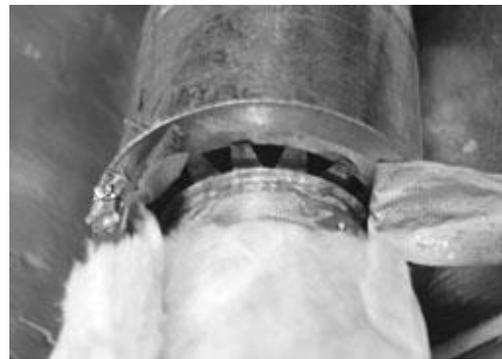
**Accelerated testing shows that fabric-backed tape with rubber adhesive tends to fall off.**
